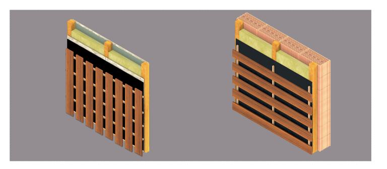
CaWrap UV 200 FR consists of a PES non-woven material and an innovative, diffusion permeable polyurethane coating, which provides long-lasting UV protection and increased fire resistance. The new CaWrap UV 200 FR meets the rising demands for increased fire protection. Driving rain or snow are effectively kept out by the insulating layer. The smooth surface of the façade membrane allows incident or infiltrating moisture to safely and securely run off.
