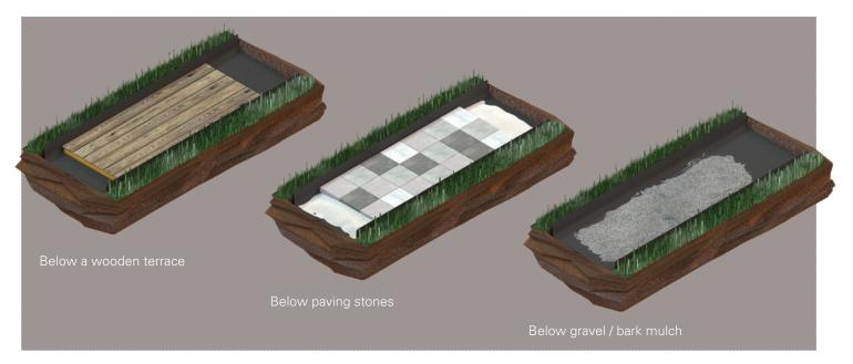
CaGround is the ideal weed-inhibiting, water permeable non-woven ground cover e.g. for applications below terrace coverings, gravel or mulch. The tried and tested geotextile is coloured black and as such does not expose open joints.
