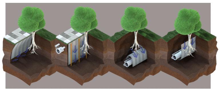
CaRoot 325 is the universal, vertically-deployed protector against roots for professional use in underground engineering, gardening, landscaping or the construction of paths. The special coating on a highly non-tear fibrous web stops the uncontrolled growth of roots. Due to this, typical problems such as damaged pipes and the necessary works in the case of uncontrolled root growth can be avoided.
