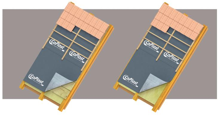
CaTop M 150 SK is a diffusion permeable, almost universally usable, sarking membrane, in accordance with DIN EN 13859-1, that has two double-sided self-adhesive strips, applied both sides. Also available without self-adhesive strips, as CaTop M 150. The multi-layer membrane is made of polypropylene non-woven fabrics separating an inner-lying functional membrane.
