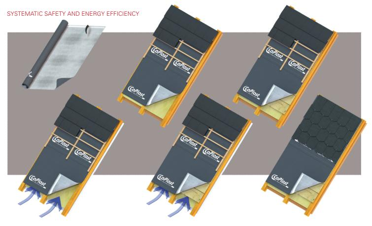
CaTop XL Strong SK is a highly tear resistant, diffusion permeable, premium sarking and underlay membrane, complying with DIN EN 13859-1. It consists of an extremely tear-resistant non-woven PES material with a polyurethane coating. CaTop XL Strong SK complies with DIN 4426 and thus can be used under large-scale tiled roofs. Available without self-adhesive strip as CaTop XL Strong.
