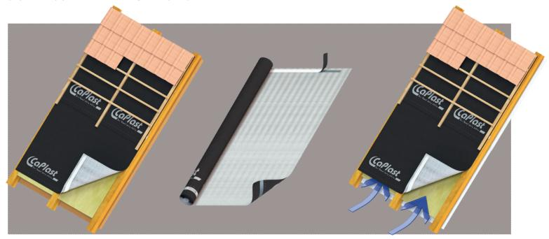
CaTop M 120 SK is a diffusion permeable, standard-compliant sarking membrane, that has two double-sided self-adhesive strips, applied both sides. Also available without self-adhesive strips, as CaTop M 120. The multi-layer membrane is made of polypropy-lene non-woven fabrics separating an inner-lying functional membrane.
