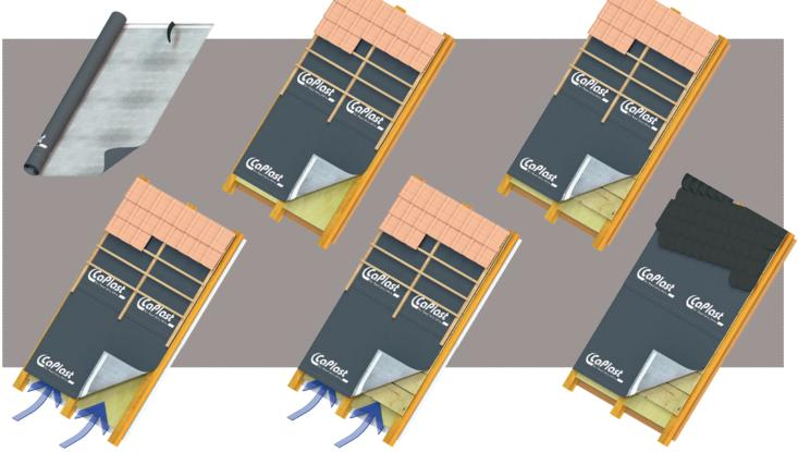
CaTop XL SK is an energy-efficient, diffusion permeable, premium sarking membrane, in accordance with DIN EN 13859-1, equipped with an integrated self-adhesive strip, and available without self-adhesive strip as CaTop XL. It consists of a non-woven PES material and an innovative, durable polyurethane coating. As a premium product, it is perfectly designed for use as a wind-resistant, rainproof sarking, underlay or temporary roof covering.
