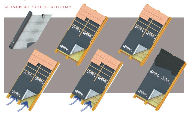
CaTop XL SK is an energy-efficient, diffusion permeable, premium sarking membrane, in accordance with DIN EN 13859-1, equipped with an integrated self-adhesive strip, and available without self-adhesive strip as CaTop XL. It consists of a non-woven PES material and an innovative, durable polyurethane coating. As a premium product, it is perfectly designed for use as a wind-resistant, rainproof sarking, underlay or temporary roof covering.
